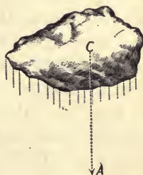
FIG. 29. — Weight is the Resultant of Innumerable Small Forces.
